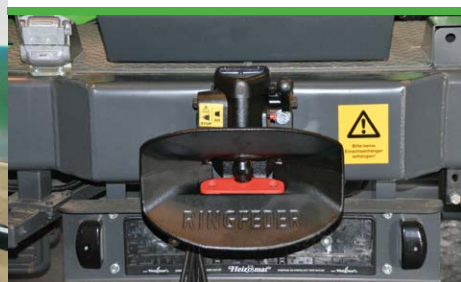
Automatic trailer coupling with compressed air connection
