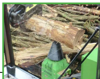
Cone splitter for pre-splitting of logs
