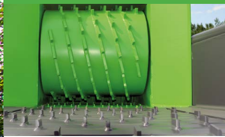
Top pressure roller Ø 520 mm
