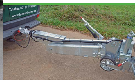
Height-adjustable drawbar for pintle hook or trailer ball
