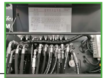
Hydraulic block incl. lever for manual operation
