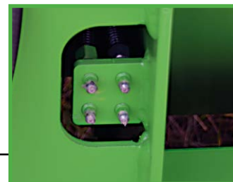
Central lubrication points easy and fast lubrication
