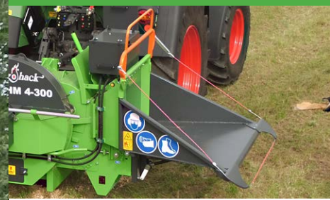
Perimeter safety cable deactivates infeed
