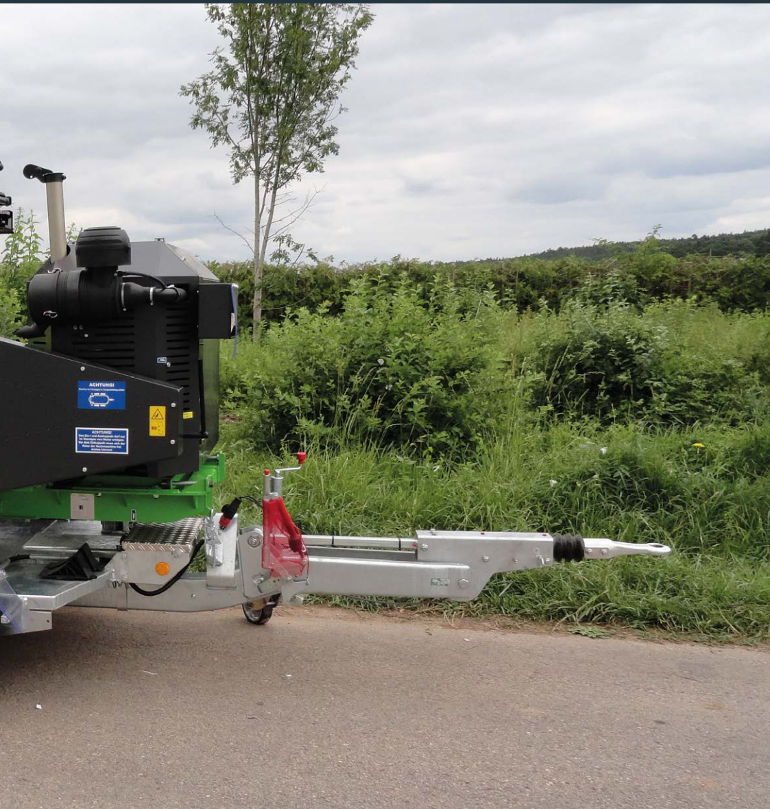
80 km/h chassis from ALKO
