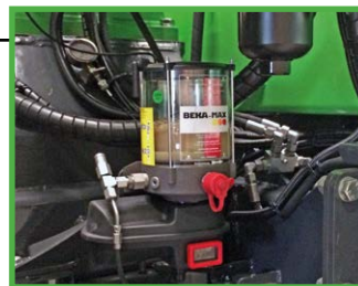
Automatic central lubrication easy and fast lubrication
