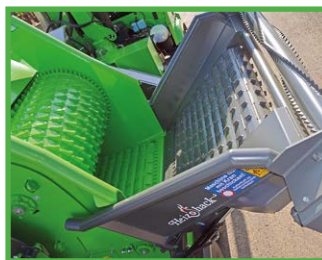
Conveyor belt at the Infeed table aggressive and powerful material infeed can be used as a funnel
