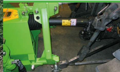
3-point-hitch extension with free wheel
