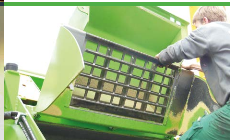
Rotor cover with extra screen
