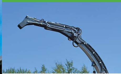
Telescoping discharge chute
