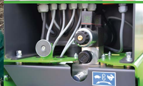
Adjustable infeed speed by hydraulic valve
