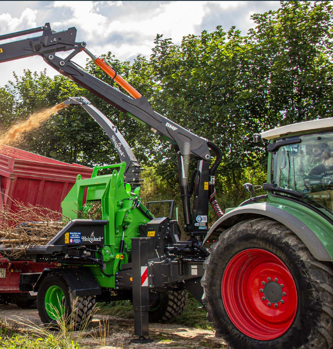
Conveyor belt infeed table
