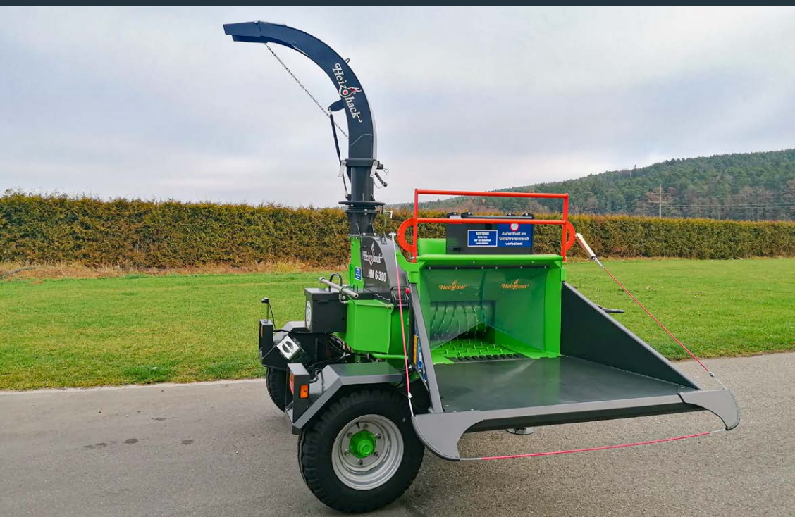
Adjustable discharge chute
