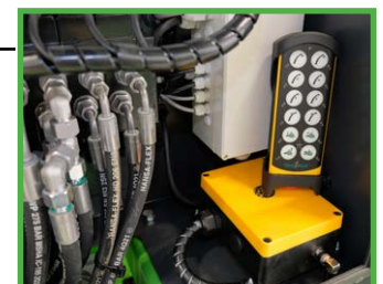
Radio remote control various hydraulic functions
