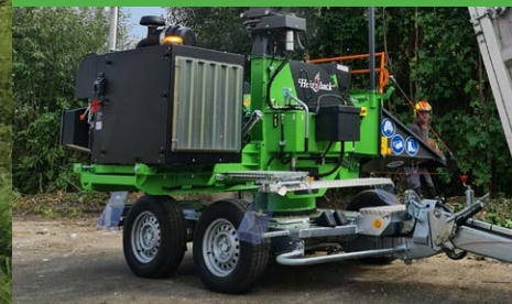
270° turntable for feeding from rear or either side
