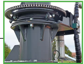
Rotating discharge chute remote control via electric motor
