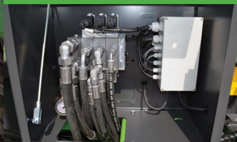
Hydraulic control block
