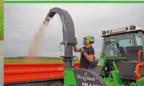
Adjustable discharge chute
