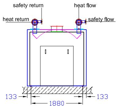
The boiler should be accessible from three sides. The discharging system should not cross the heating room.
